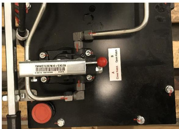
Figure 11. Selector for manual operation.
