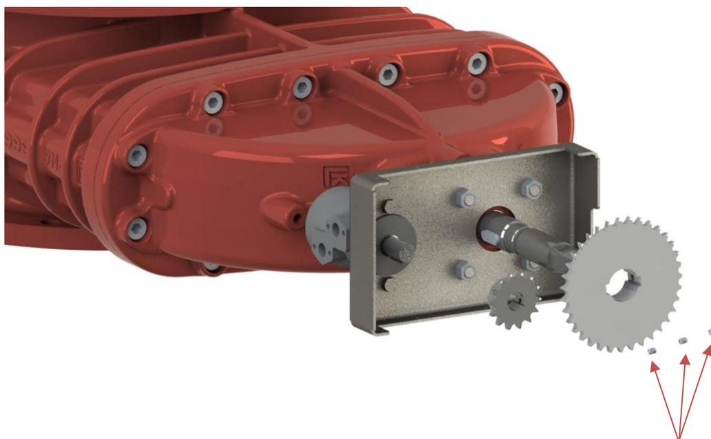
6. Mount the open chain around the sprockets and lock it in place.
