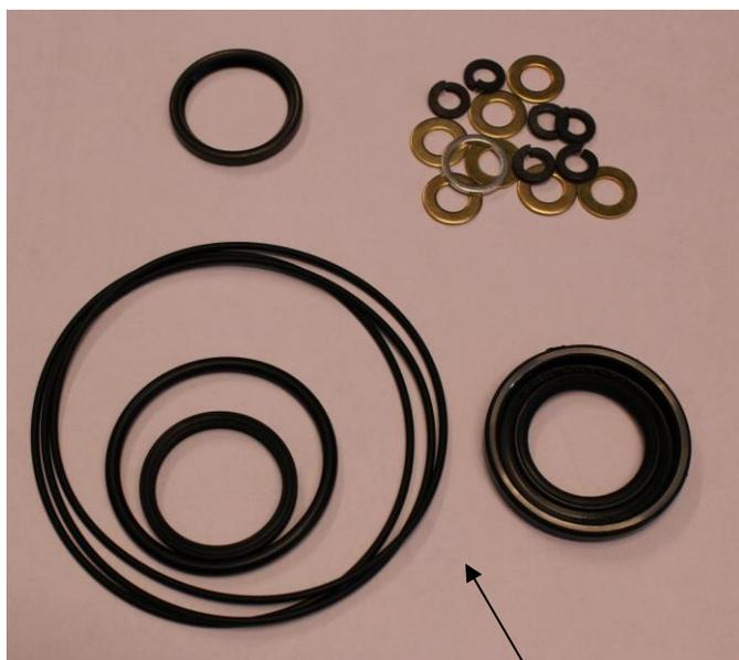
Figure 19. Service kit – hydraulic motor.
