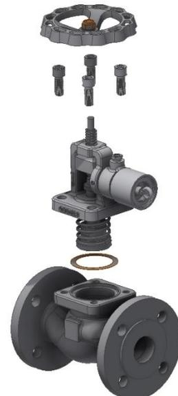
10. Re-assemble the stem with disc and spring into the bonnet using the new setting nut. Don't forget the indication washer.
